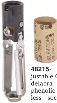
48209- Candelabra base phenolic keyless socket with (fixed) 1/8 IP hickeys. 3" overall ht. U.L. listed.
