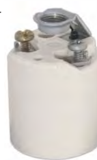
48104- 660W-250V, Heavy duty unglazed porcelain keyless standard-size socket. Has 1/8F detachable hickeys. U.L. & CSA listed.
