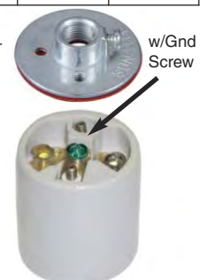
NEW! 48303- E26, 660W-250V Keyless Porcelain 3-Terminal Socket with Ground Screw, measures 1 1/2" wide by 2 1/16" ht. Comes with 1/8 IP threaded metal cap. UL Listed.
