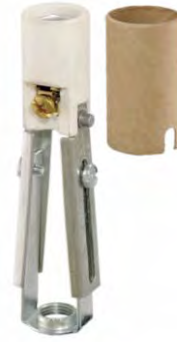
Adj. Porcelain Candelabra size keyless socket with 1/8 IP hickeys. U.L. listed 48317- adjusts from 3 3/8" to 4 11/16" 48318- adjusts from 4 11/16" to 6"
