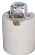
48301- 660W-250V, Heavy duty unglazed porcelain keyless standard-size socket. Has 5/8" detachable 1/8F hickeys. U.L. & CSA listed.
