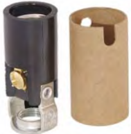
48312- Candelabra size phenolic keyless sockets w/fixed 1/8 IP hickeys. 3/8" hickey (1 3/4" overall ht.), U.L. listed
