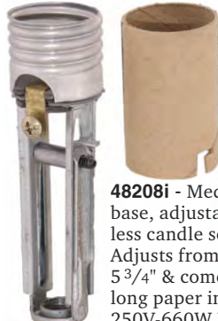
48208 - Medium base, adjustable keyless candle socket. Adjusts from 4" to 5 3/4" & comes w/a long paper insulator. 250V-660W UL CSA
