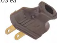
Cooper Brand Heavy Bakelite style plug w/brass prongs & screw-terminal attachment. Good for STP-2 & SVT round lamp cord.
