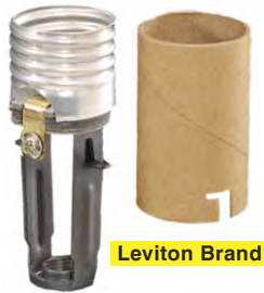
48226- Medium base, keyless candle socket. 3" ht. with 1/8 IP hickeys, comes w/a long paper insulator. 250V-660W UL CSA.
