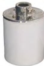
48302- Glazed porcelain keyless standard-size socket w/high heat resistance. Has bottom insulator, 1/8 IP female metal cap & set screw. 660W - 220V, U.L. & CSA listed.
