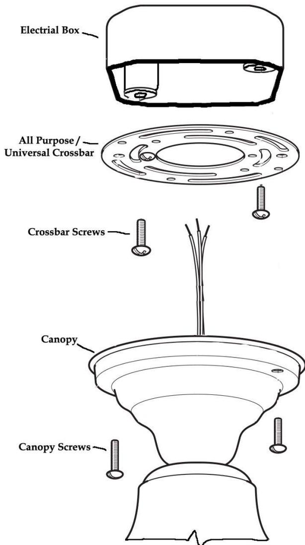
1) Before removing an old fixture or installing a new one, shut off the power to the circuit by turning off the breaker or removing the fuse. Just turning the light switch off will not protect against possible electrical shock.
